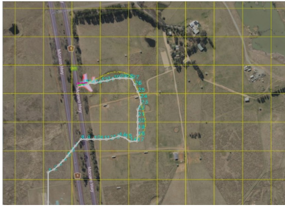
Fig. 7. Comparison between the planned Hybrid A* path and the actual flight trajectory executed by the UAV in the Gazebo physics simulation.
